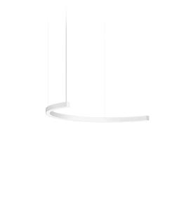
Suspension lighting fixture for interiors, with direct light emission. Bended extruded aluminium structure in white, black or mat brass polyacrylic paint. Extruded polycarbonate diffuser with opaline finish. Galvanized sheet metal end caps in polyacrylic paint. Suspension kit with griplocks and 2m (78,7") long steel cables. 2,2m (86,6") long power cable in transparent PVC. Power canopy with pickled sheet metal ceiling bracket and covering in white polyacrylic paint.
